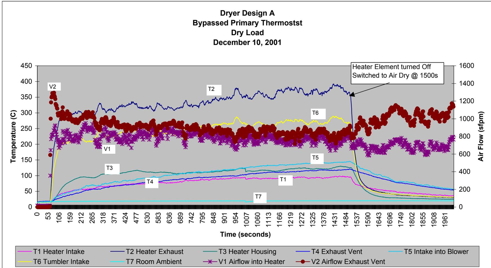
Figure 17. Dryer Design A – Primary Thermostat Bypassed
