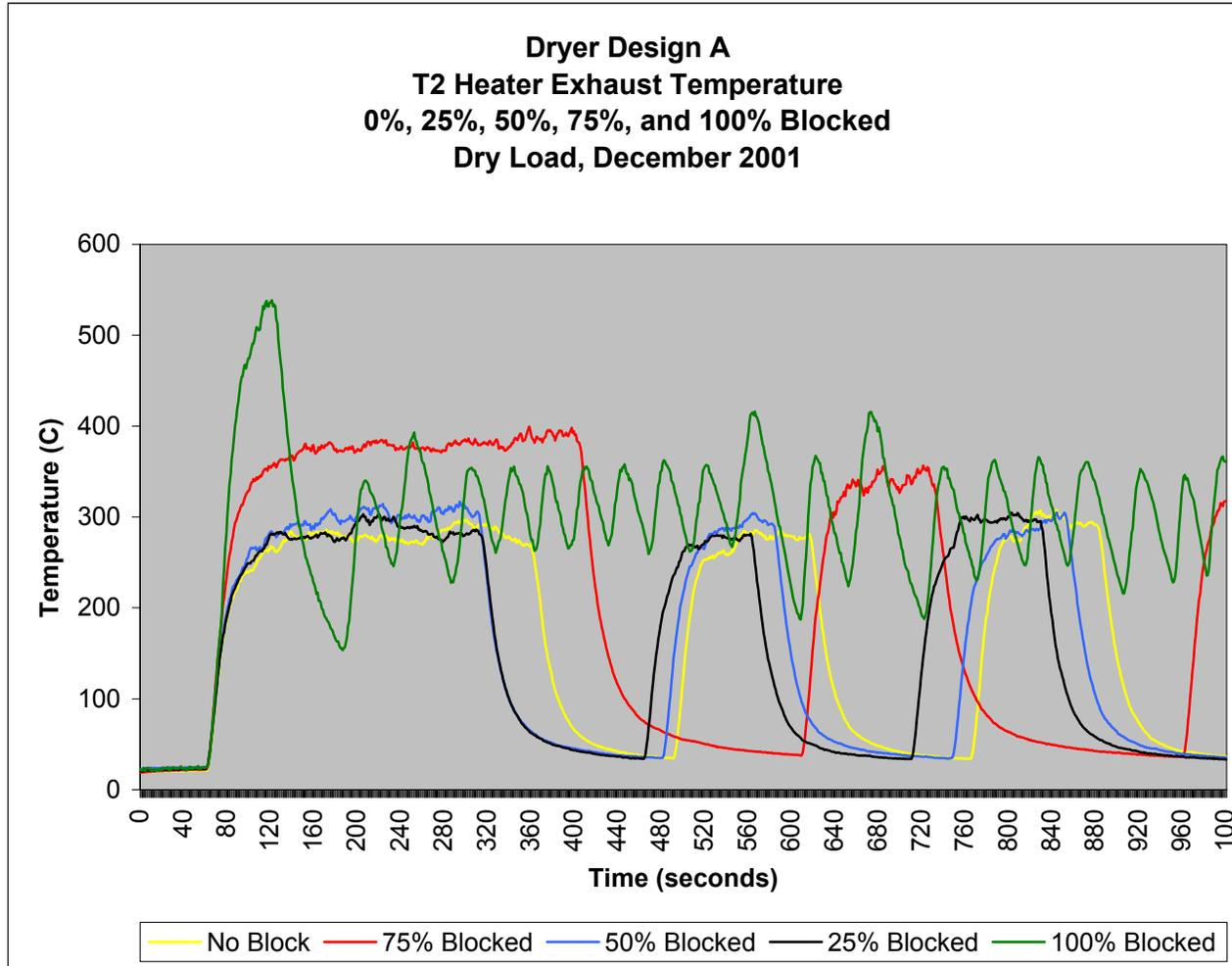
Figure 12. Dryer Design A – T2 Heater Exhaust Comparison
