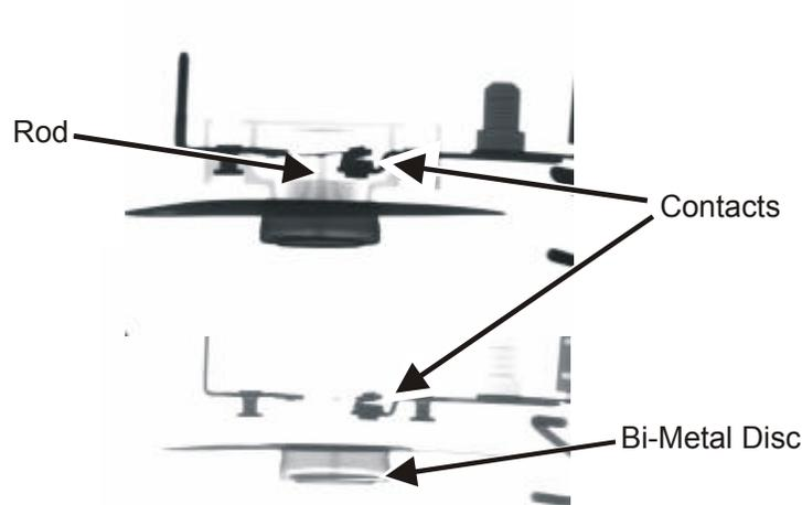
Figure 106. X-ray Images of High-Limit Thermostat 2 (HLT2)
