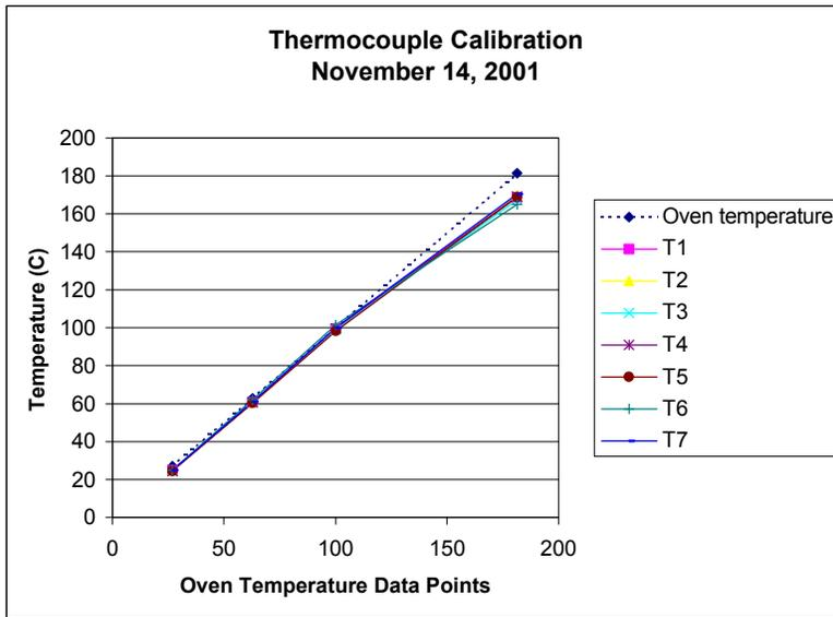
Figure 5. Thermocouple Response Before Task 2 Testing
