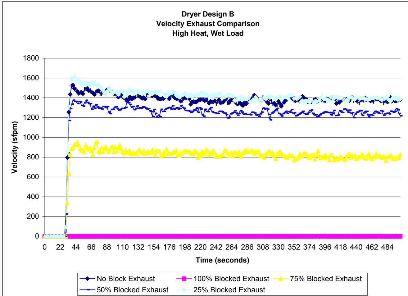
Figure 24. Dryer Design B – Exhaust Vent Air Velocity
