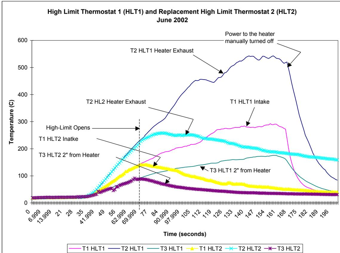
Figure 100. Failed Thermostat compared to a Replacement Thermostat
