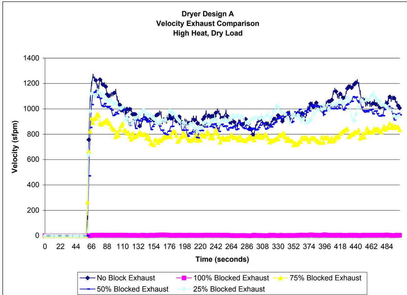
Figure 14. Dryer Design A – Exhaust Air Velocity
