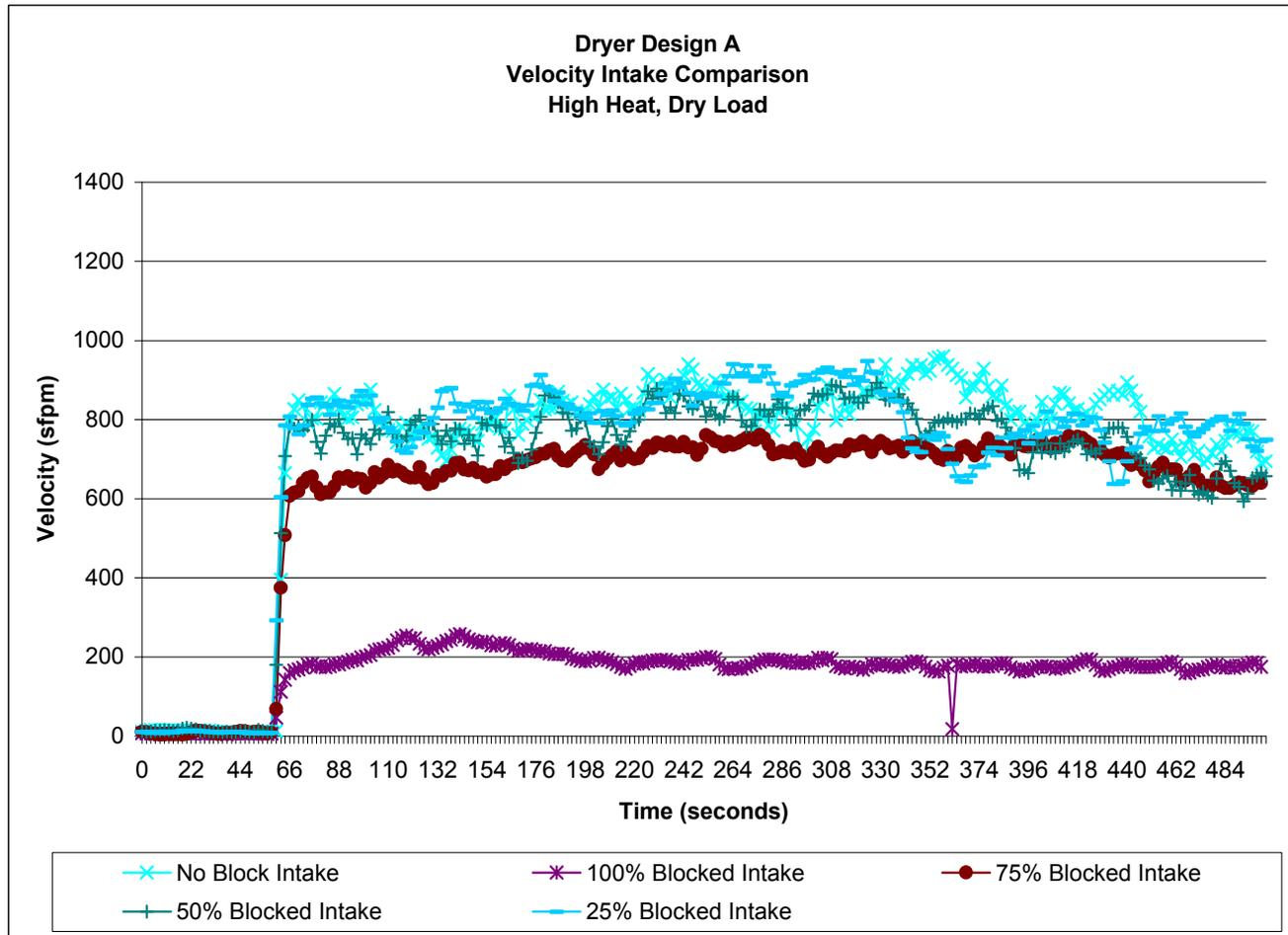
Figure 13. Dryer Design A – Intake Air Velocity
