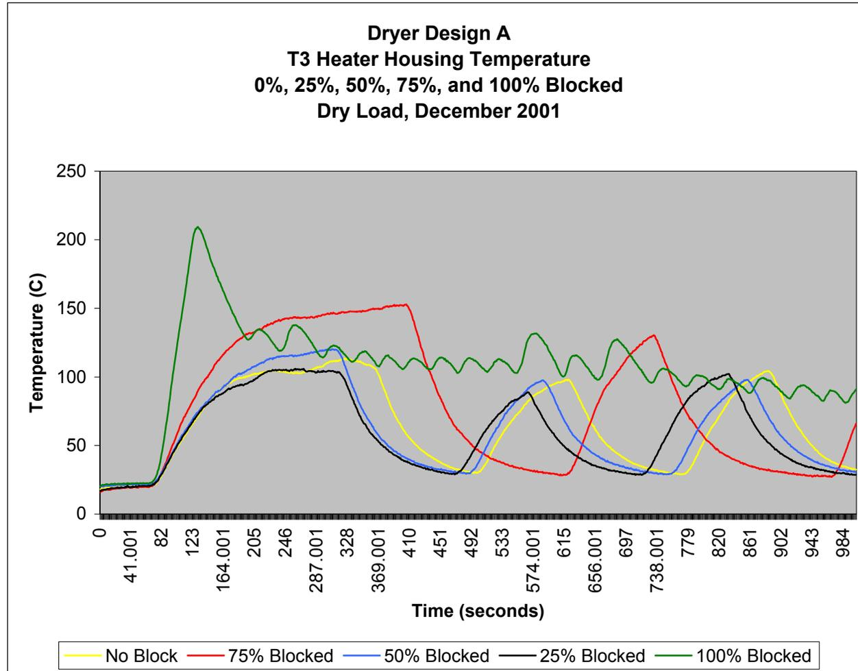
Figure 11. Dryer Design A – T3 Heater Housing Comparison
