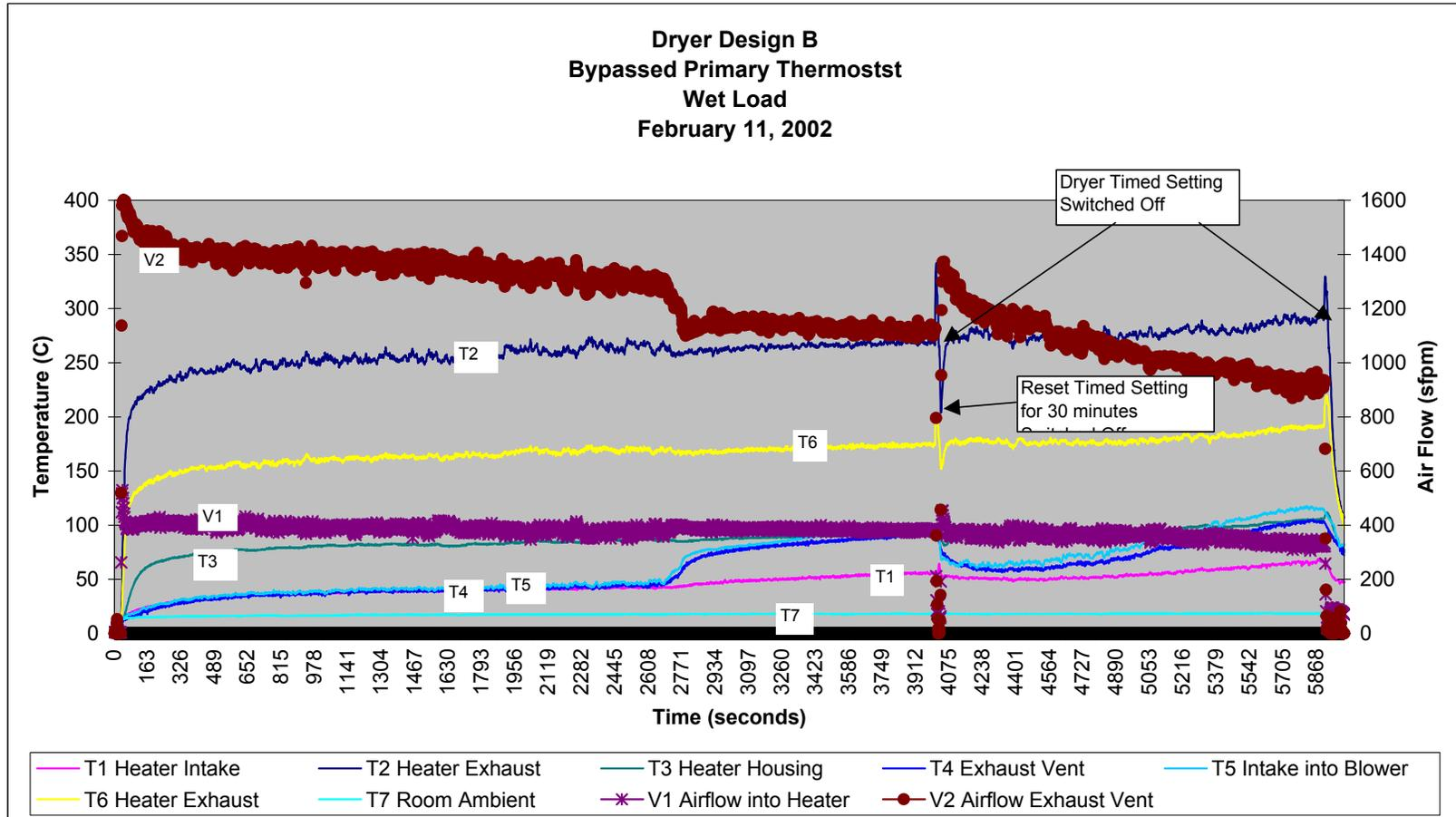
Figure 26. Dryer Design B – Primary Thermostat Bypassed
