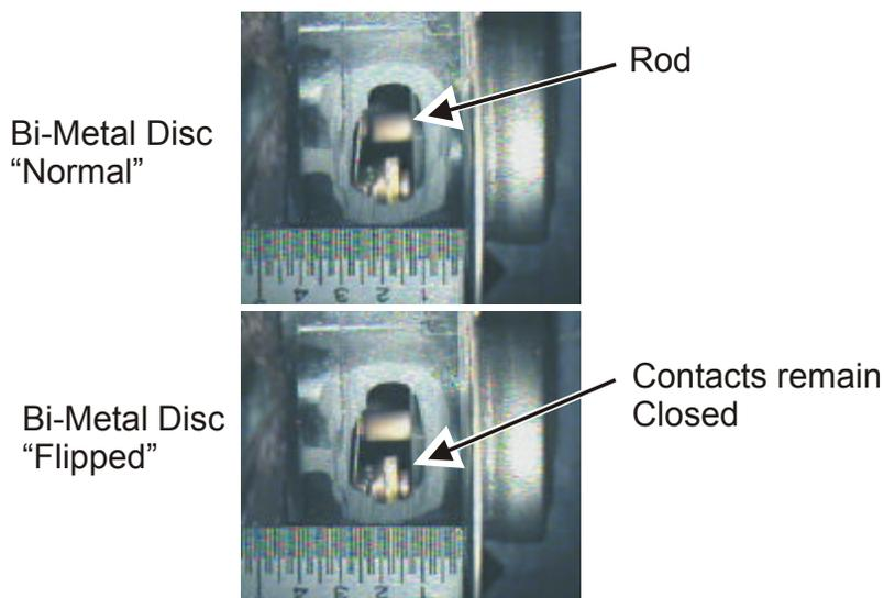
Figure 111. Second Failed High Limit Thermostat, HLT2
