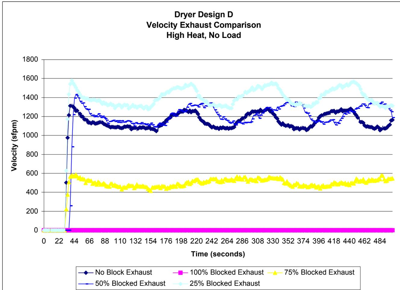
Figure 43. Dryer Design D – Exhaust Vent Air Velocity
