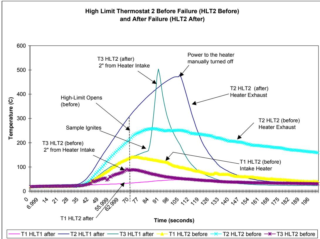
Figure 105. High-Limit Thermostat 2 (HLT2) before and after Failure
