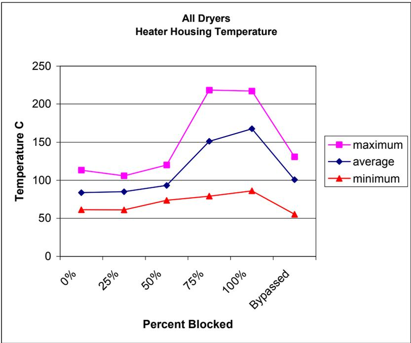
Figure 78. Heater Housing Temperature
