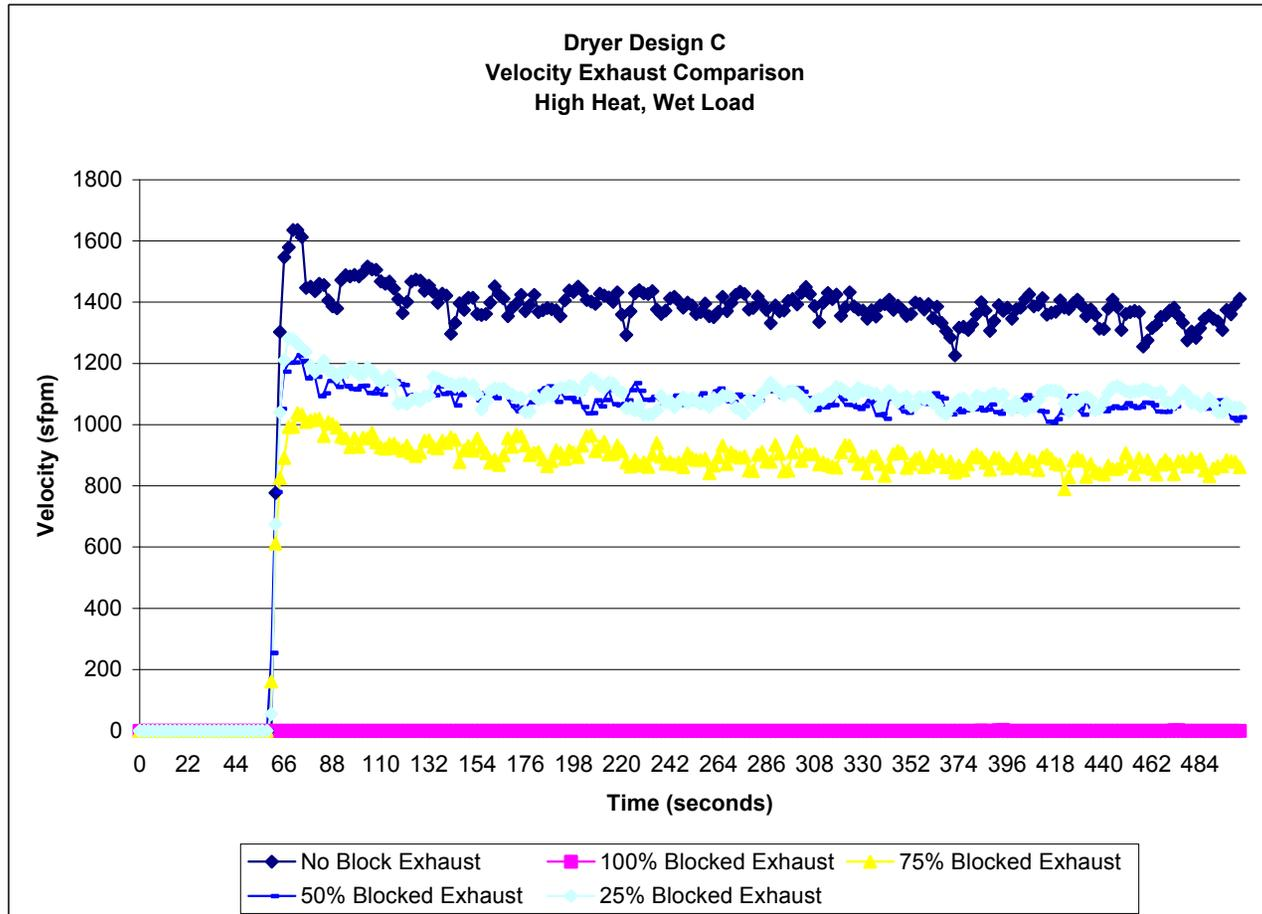
Figure 33. Dryer Design C – Exhaust Vent Air Velocity
