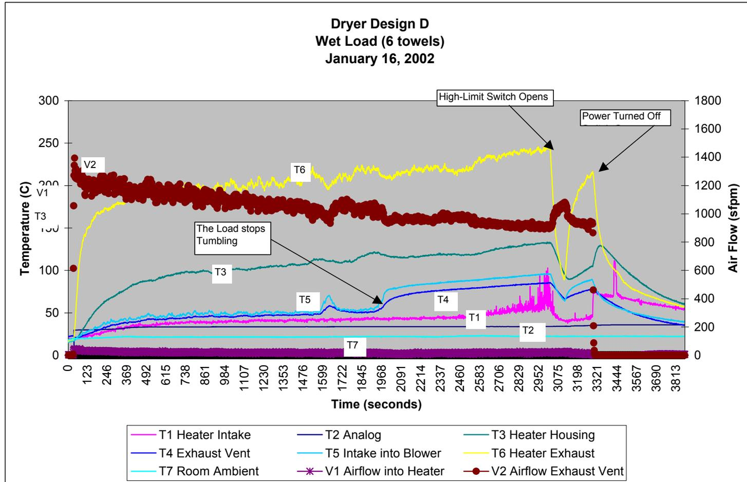
Figure 45. Dryer Design D – Primary Thermostat Bypassed
