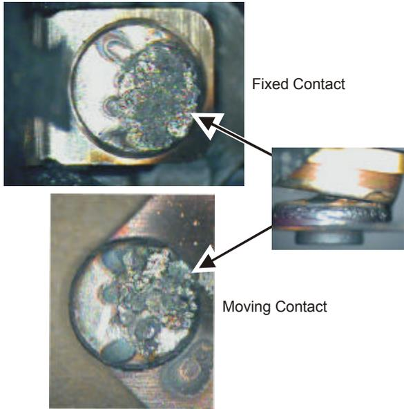
Figure 103. Contact Pads for High-Limit Thermostat 1 (HLT1)
