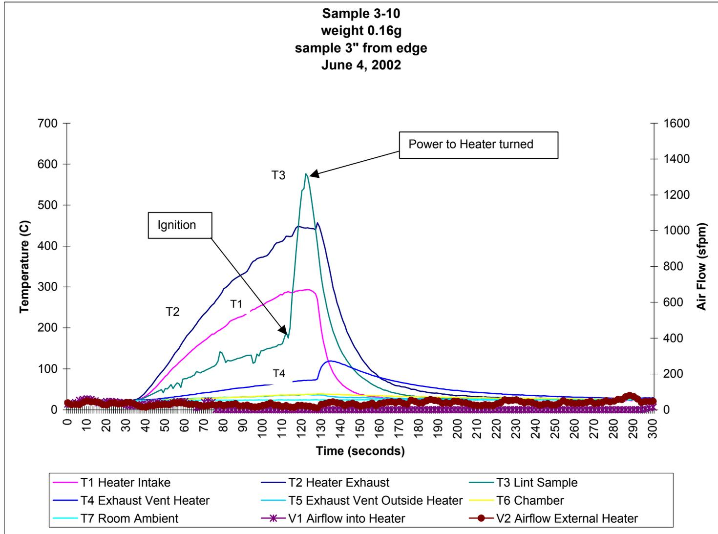
Figure 66. Sample s3-10 – Thermocouple and Airflow Data
