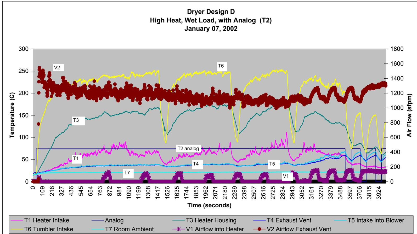
Figure 39. Thermocouple, Airflow and Relay (T2 Analog) Measurements
