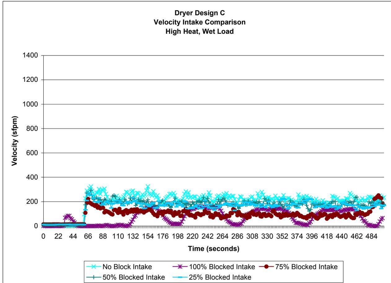
Figure 32. Dryer Design C – Intake Air Velocity
