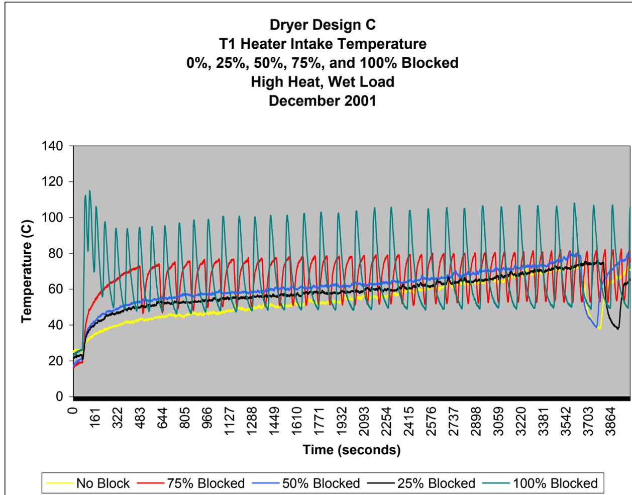
Figure 29. Dryer Design C – T1 Heater Intake Comparison
