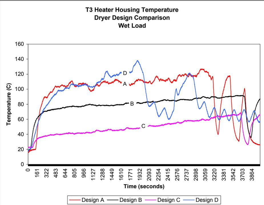
Figure 72. Dryer Design Comparison for T3, Heater Housing
