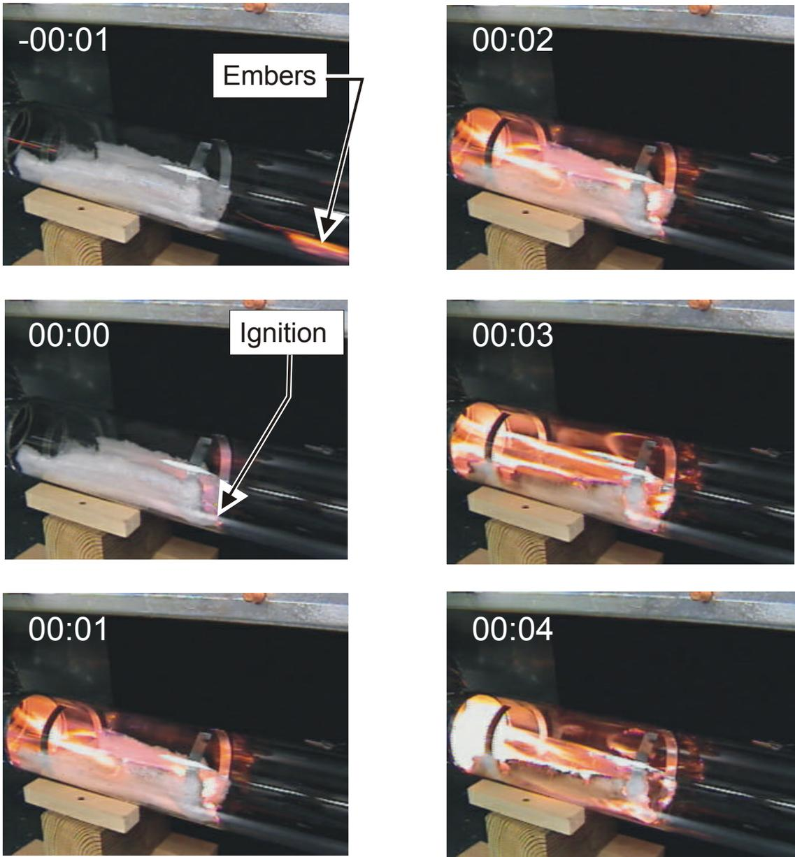
Figure 69. Target Sample Igniting During Test 1
