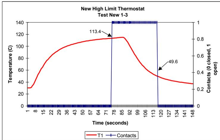
Figure 110. Thermocouple Data for the New High-Limit Thermostat
