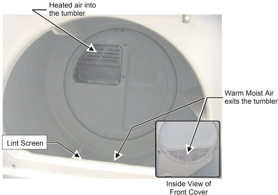
Figure 27. Dryer Design C – Airflow through the Tumbler
