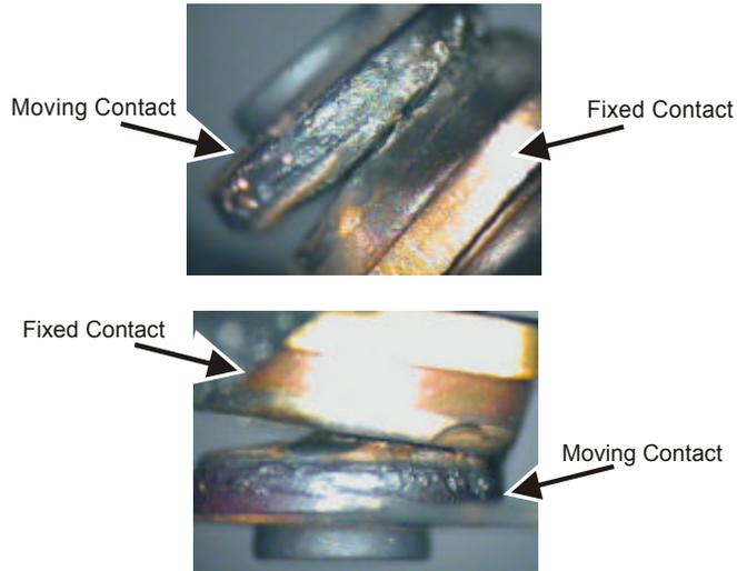
Figure 102. Contacts for High-Limit Thermostat 1 (HLT1)
