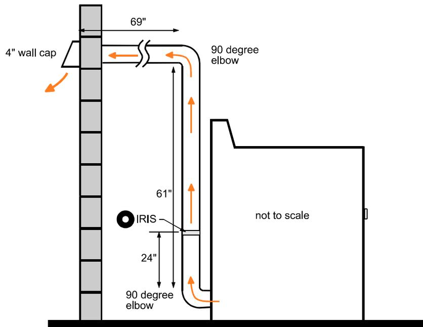
Figure 4. Exhaust Vent Setup
