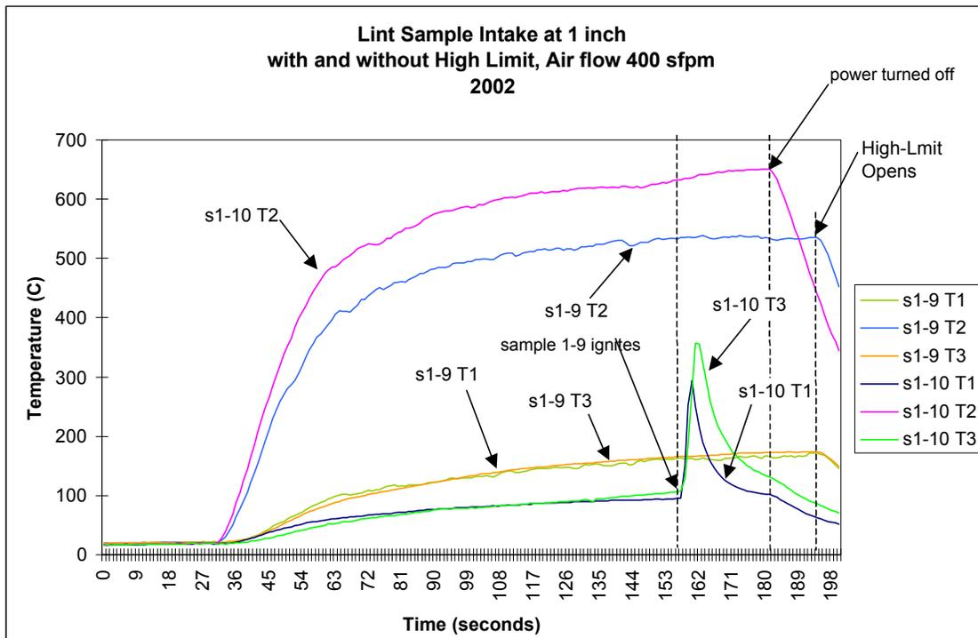
Figure 98. Samples Tested at 1 Inch, With and Without High-Limit Thermostat
