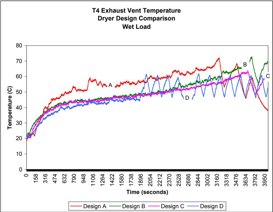
Figure 74. Dryer Design Comparison for T4, Exhaust Vent
