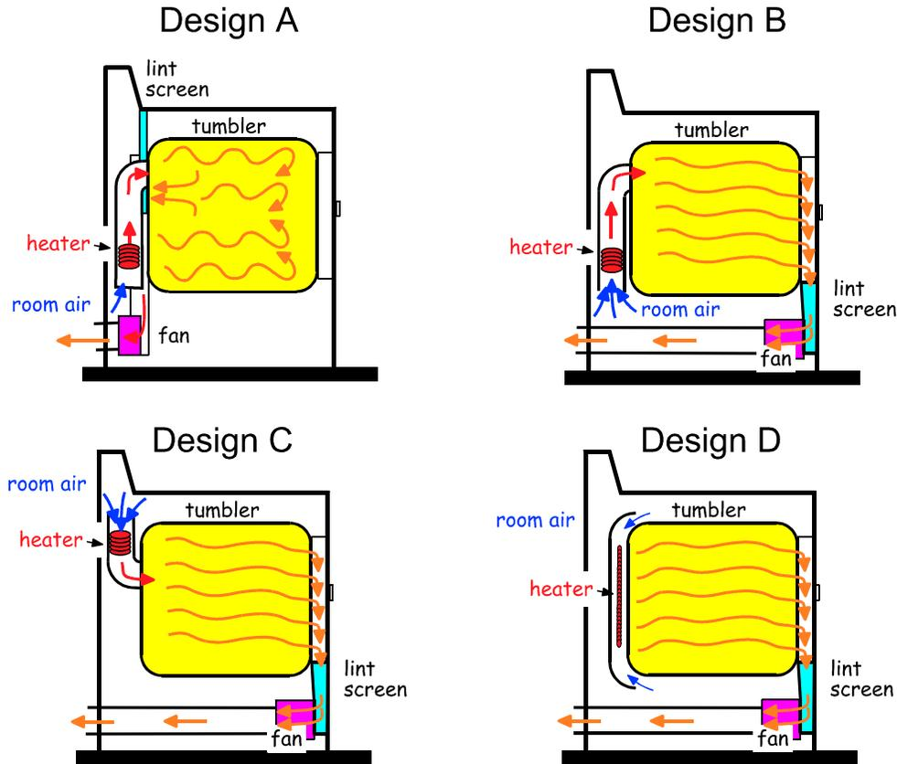
Figure 1. Dryer Design Characteristics
