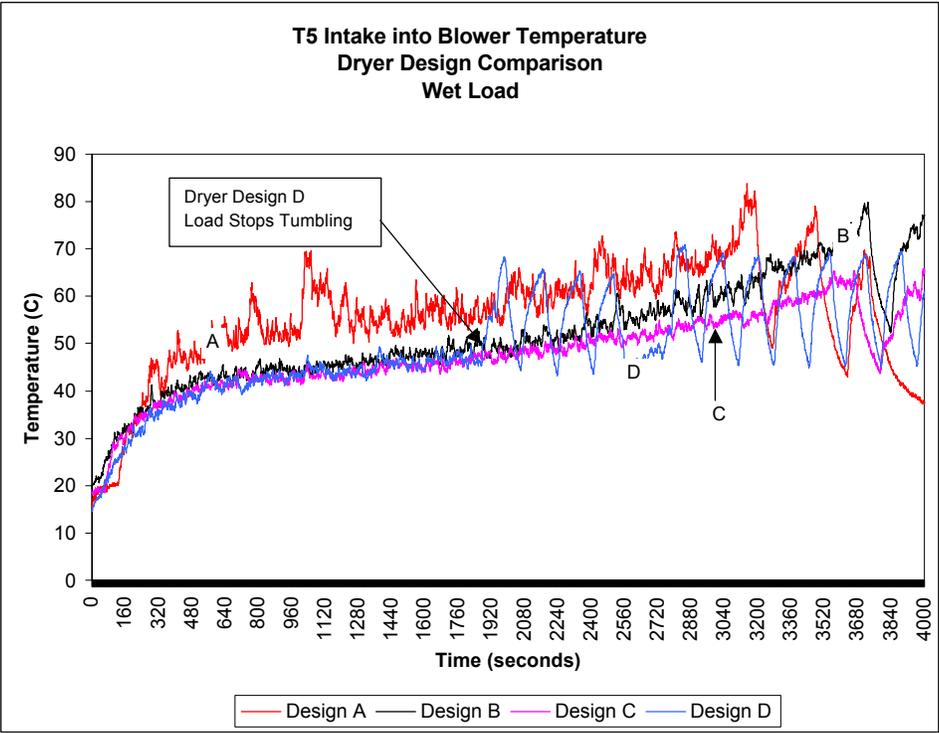
Figure 73. Dryer Design Comparison for T5, Blower Intake
