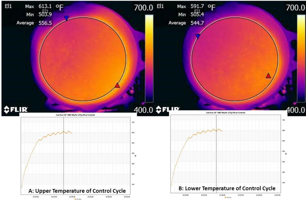
**Figure 40: A: Upper Temperature of the Cycle (Left) and B: Low Temperature of the Cycle (Right), IR Temperature Profile for 10 inch Cast Iron Pan; 18,500 Btu/hr. Burner Rate; Controls Active**
