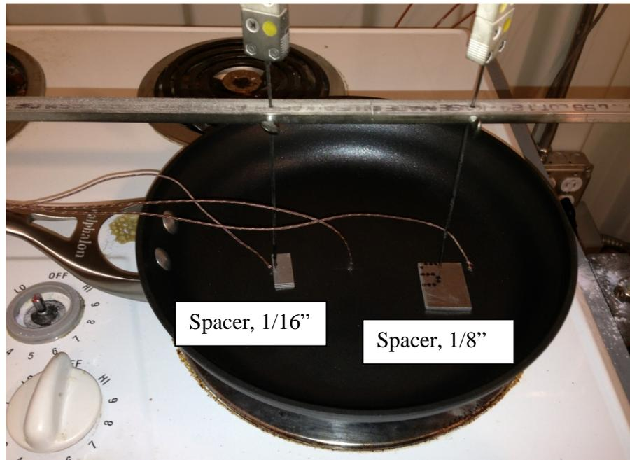
**Figure 10: Use of Spacers to Locate Thermocouples in Oil**
