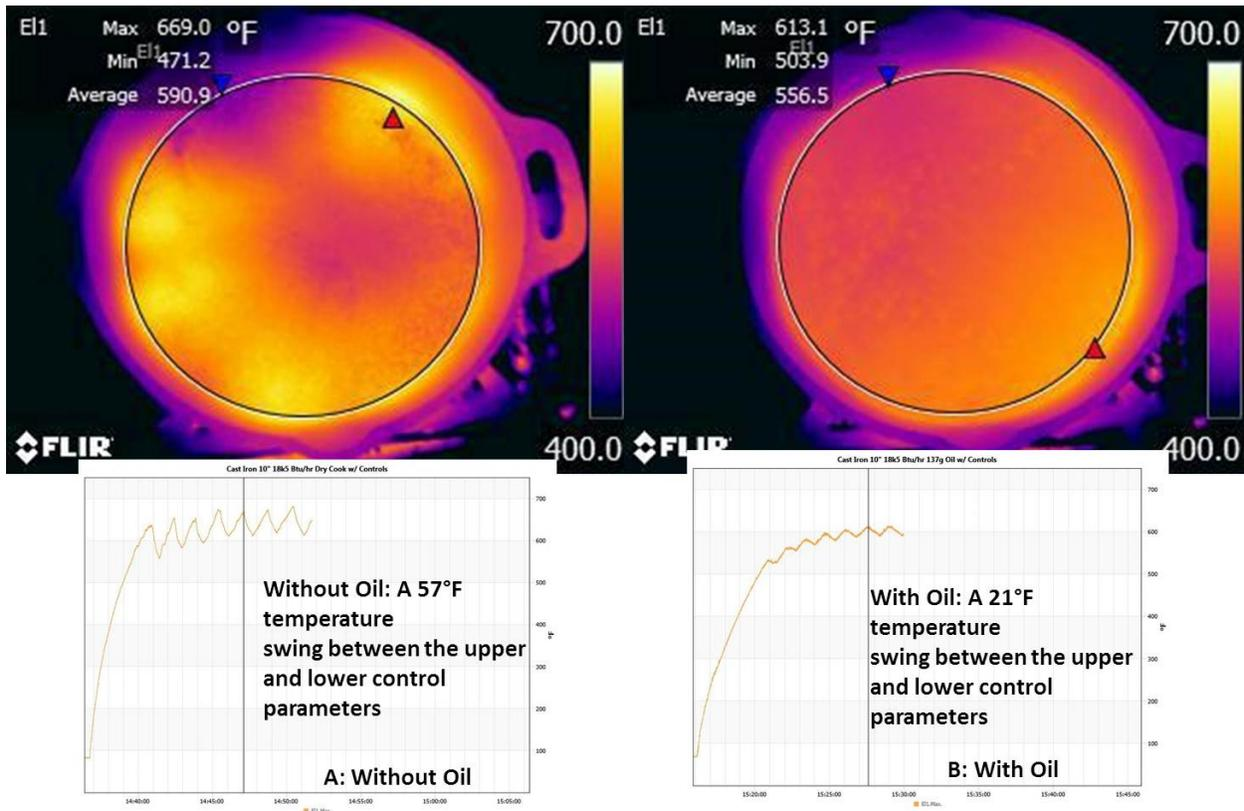
**Figure 38: A: Without Oil (Left) and B: With 150 mL Oil (Right), IR Temperature Profile for 10-Inch Cast Iron Pan; 18,500 Btu/hr. Burner Rate; Controls Active**
