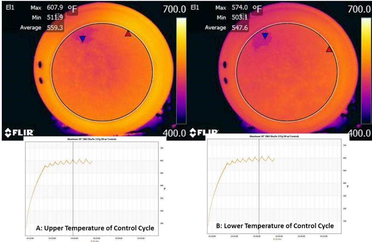
**Figure 39: A: Upper Temperature of the Cycle (Left) and B: Low Temperature of the Cycle (Right), IR Temperature Profile for 10-inch Aluminum Pan; 18,500 Btu/hr. Burner Rate; Controls Active**
