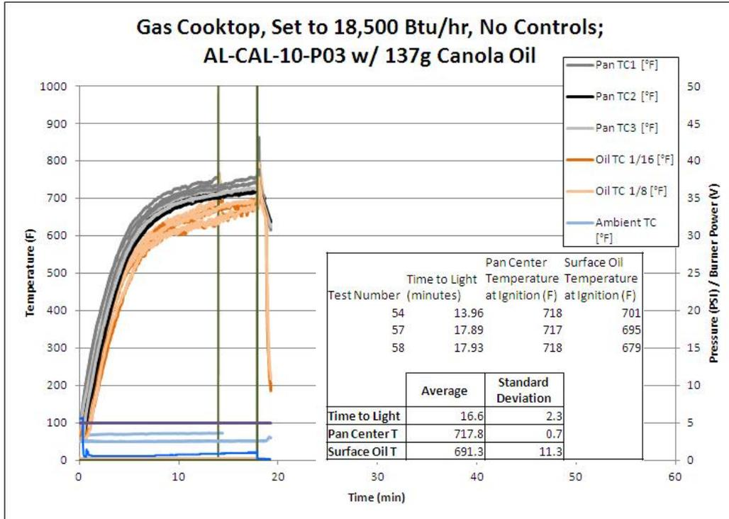
Figure 14: Aluminum Pan Repeatability Tests: 150mL (137g) of Oil; 10-Inch Pan
