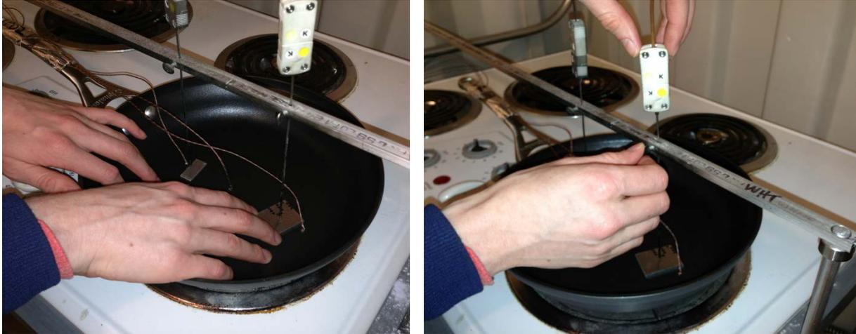
**Figure 11: Locating Thermocouples**
