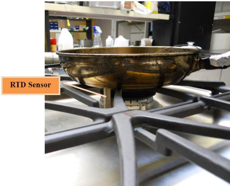
**Figure 3: RTD Sensor Being Engaged by a Stainless Steel Pan**
