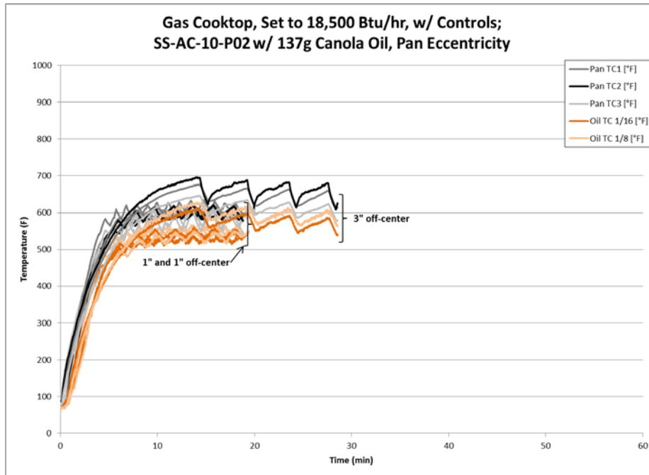
Figure 30: Summary of Oil Temperatures for Pan Eccentricity Tests
