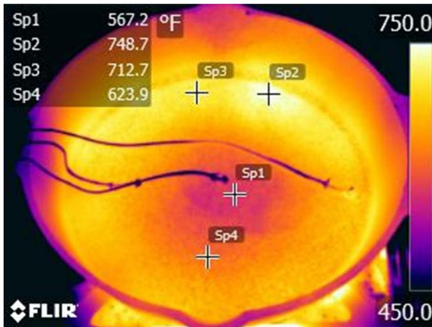
Figure 36: Temperature Profile Across a Cast Iron Pan at Power Boil Setting (18,500 Btu/hr.)
