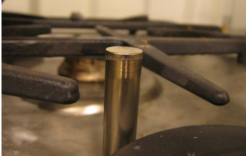
**Figure 4: Pan Bottom Temperature Sensor**
