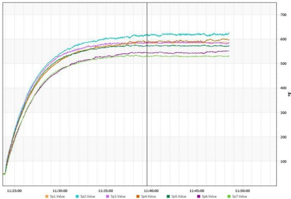
Figure 32: Temperature Distribution Across Aluminum Pan on a Standard Burner
