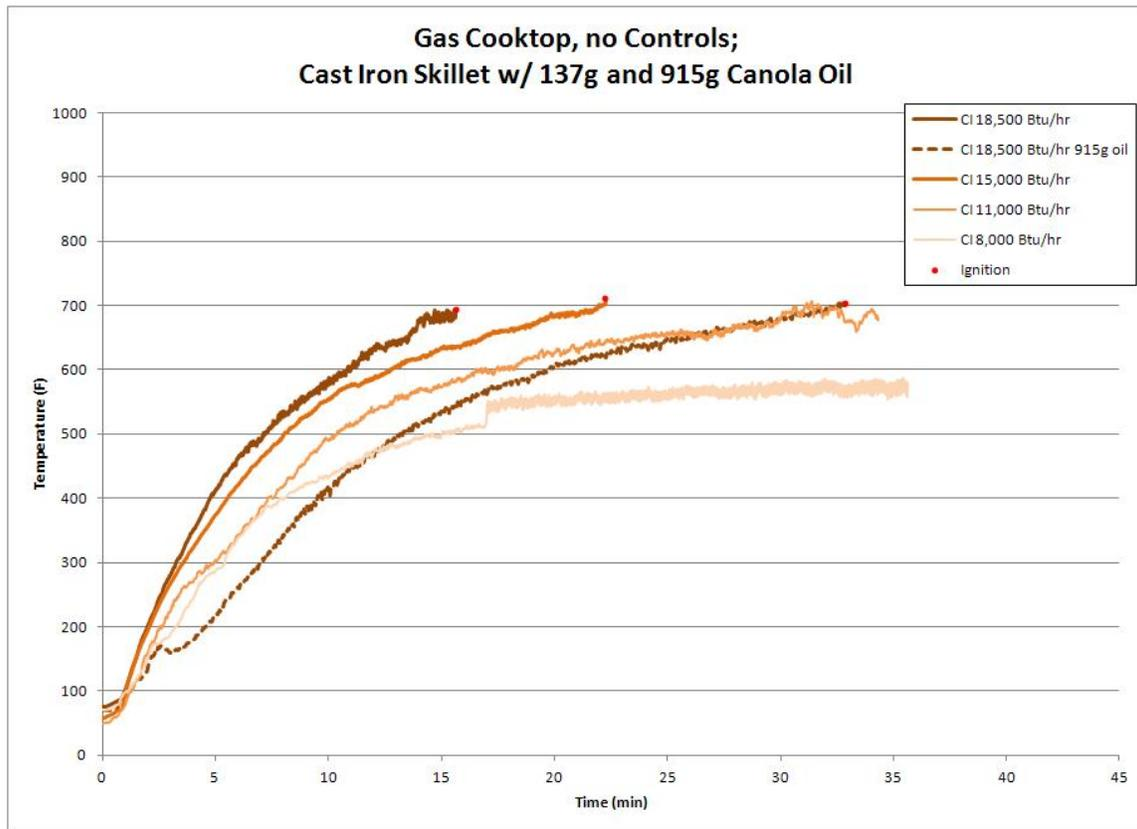
Figure 20: Surface Oil Temperature Profiles for Cast Iron Pans
