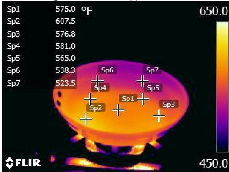
Aluminum 10" Front Left Burner (no sensor) set to 8000 Btu/hr
