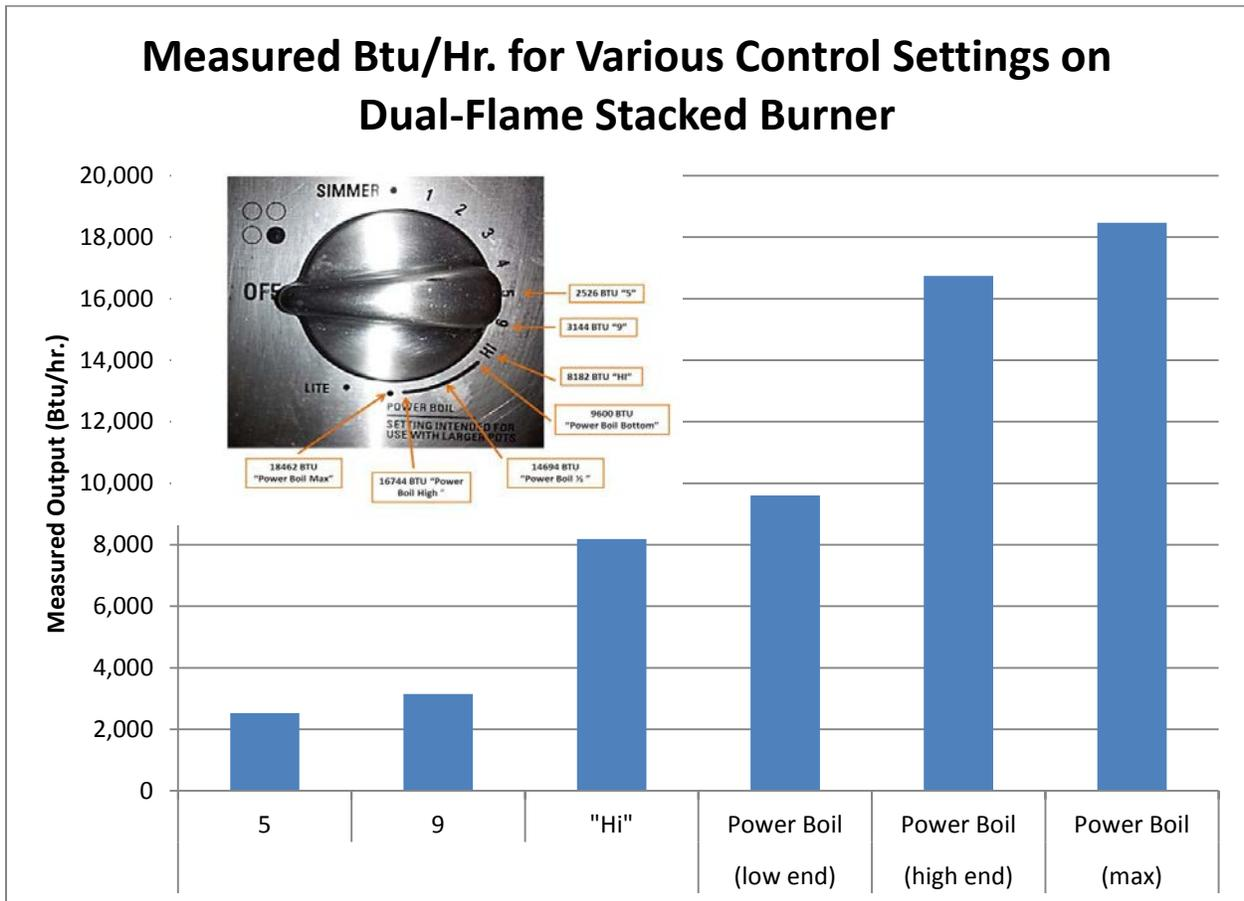
**Figure 2: Heat Rate Calibration for the Gas Burner Tested**
