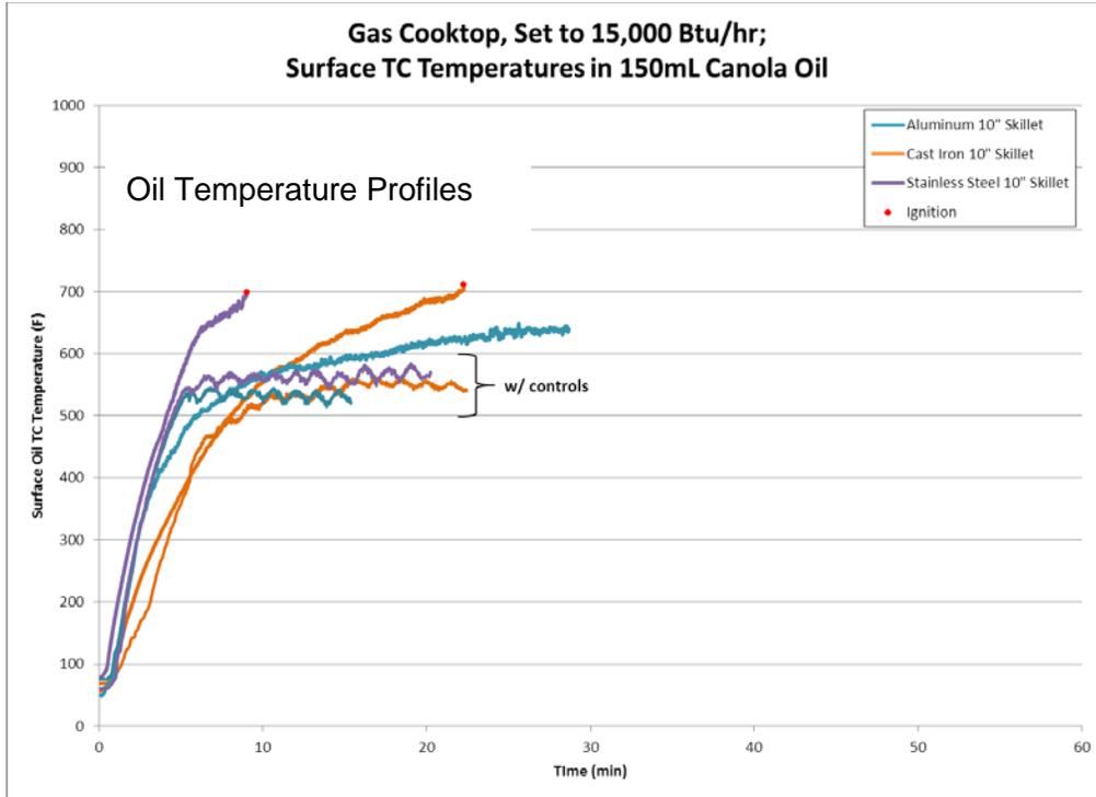
Figure 25: Comparison of Oil Temperature Profiles for Baseline and Control System Tests (15,000 Btu/hr.)
