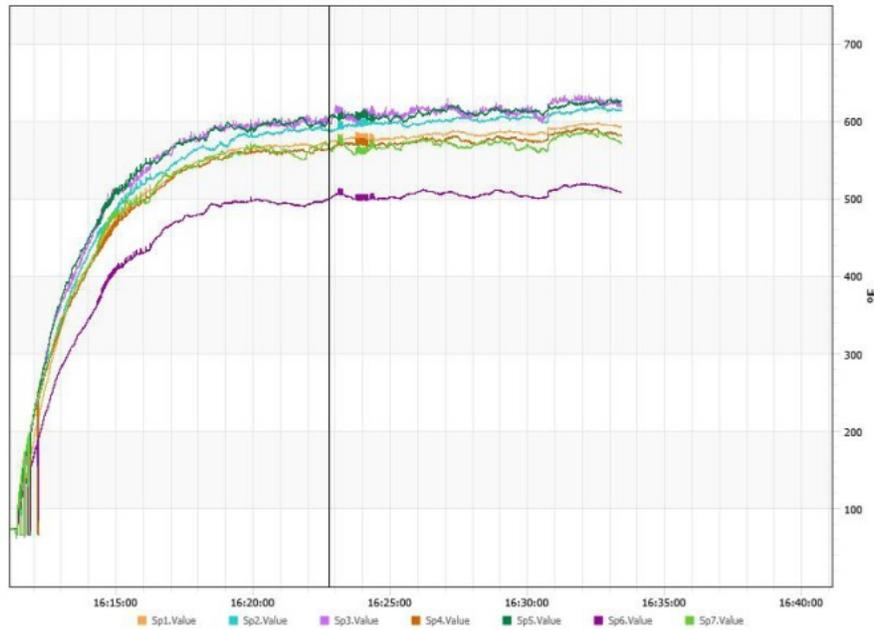
**Figure 31: Temperature Profile in Aluminum Pan on High Setting (8,000 Btu/hr.)**
