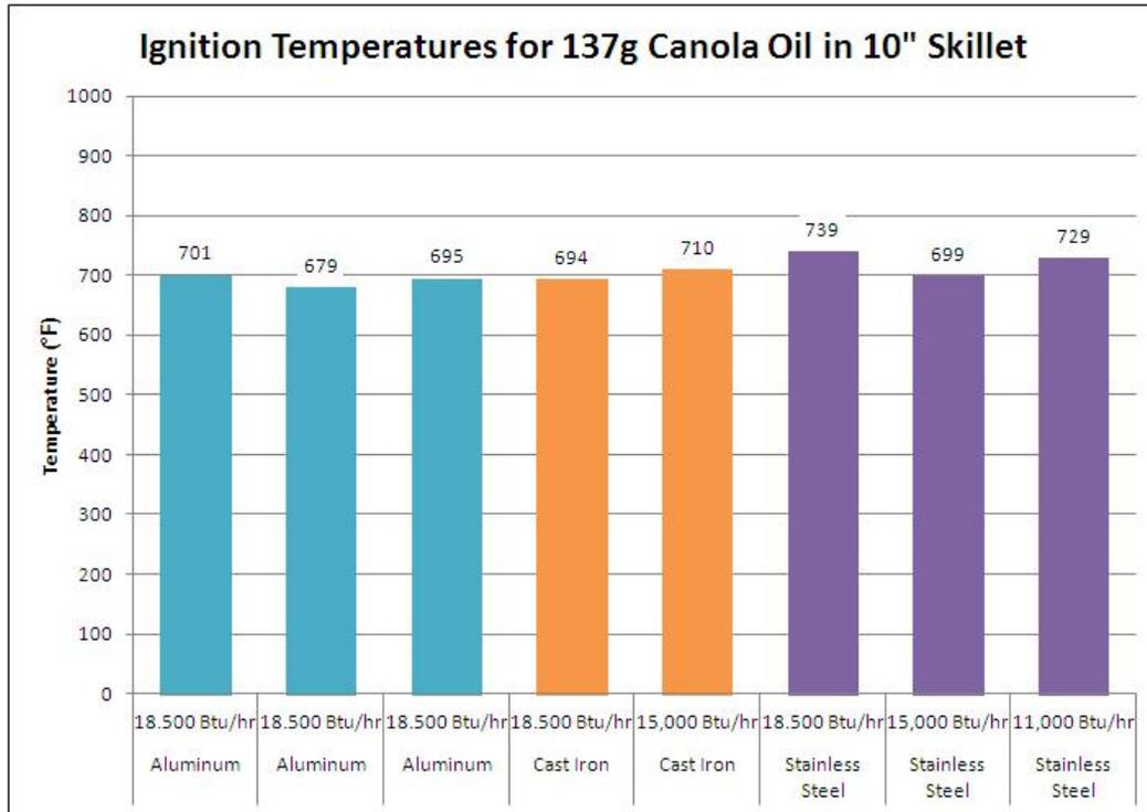
Figure 22: Oil Ignition Temperatures for 150 ml Oil
