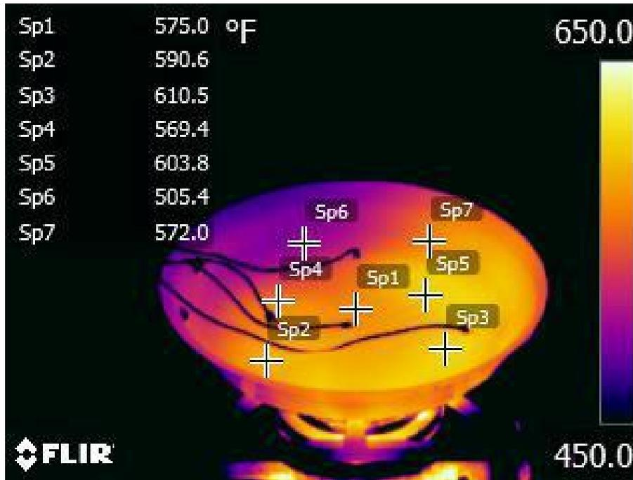
Aluminum 10" Front Right Burner (with Sensor) Set to 8000 Btu/hr
