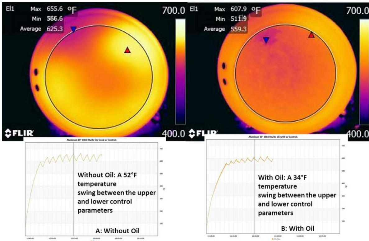
**Figure 37: A: Without Oil (Left) and B: With 150 mL Oil (Right), IR Temperature Profile for 10 inch Aluminum Pan; 18,500 Btu/hr. Burner Rate; Controls Active**
