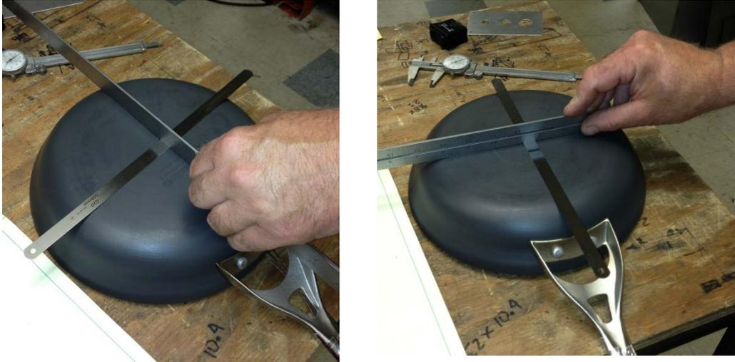
**Figure 9: Pan Warpage Measurement**
