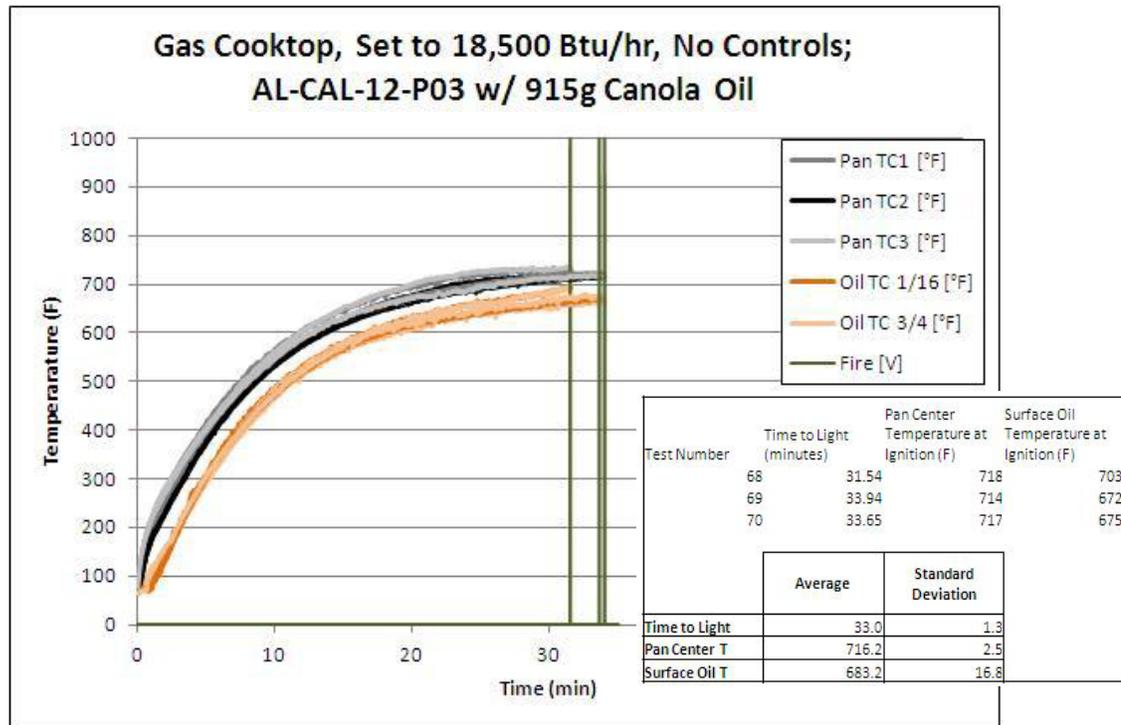
Figure 15: Aluminum Pan Repeatability Tests: 1,000ml (915g) of Oil, 12-inch Pan
