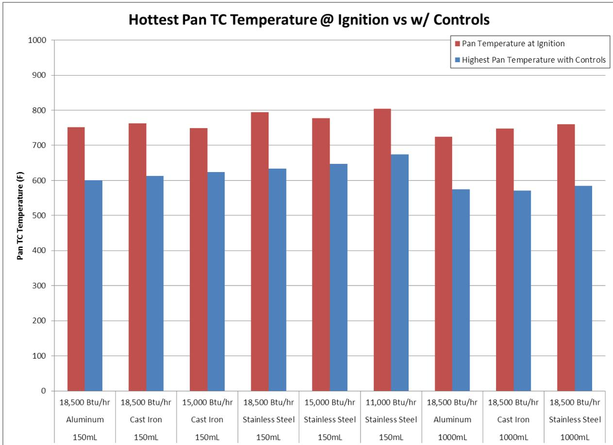
**Figure 24: Maximum Pan Temperatures with and without Controls**
