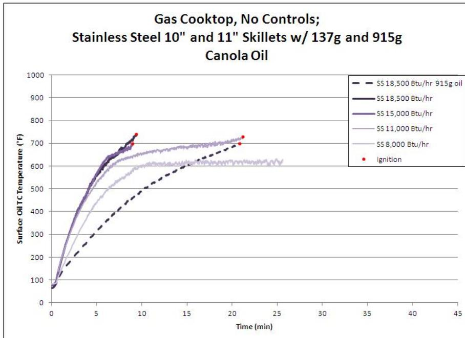
**Figure 19: Surface Oil Temperature Profiles for Stainless Steel Pans**
