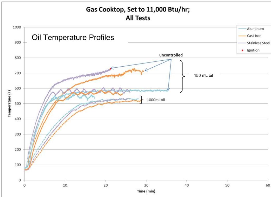
Figure 26: Comparison of Oil Temperature Profiles for Baseline and Control System Tests (11,000 Btu/hr.)
