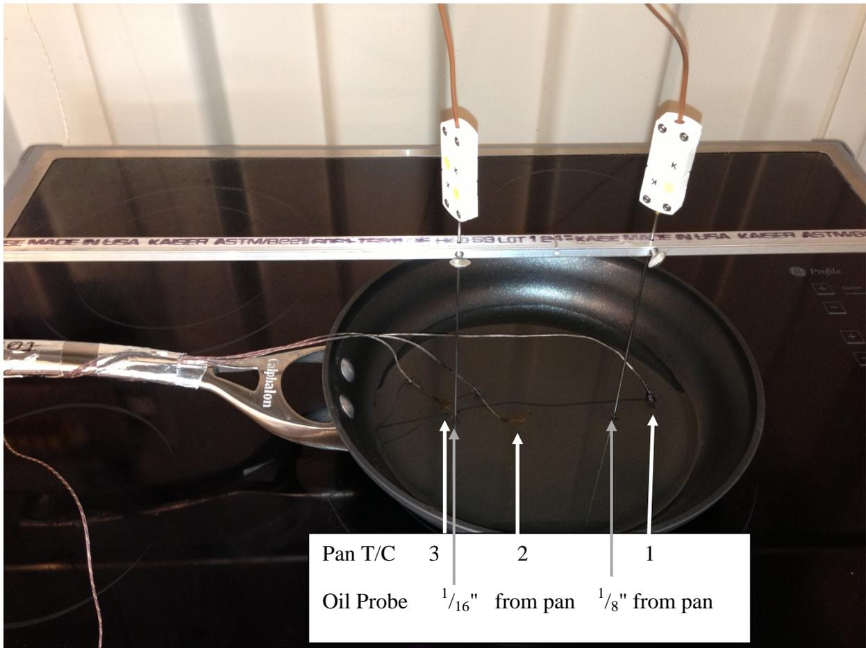
Figure 13: Locations of All Thermocouples in Pans and Oil
