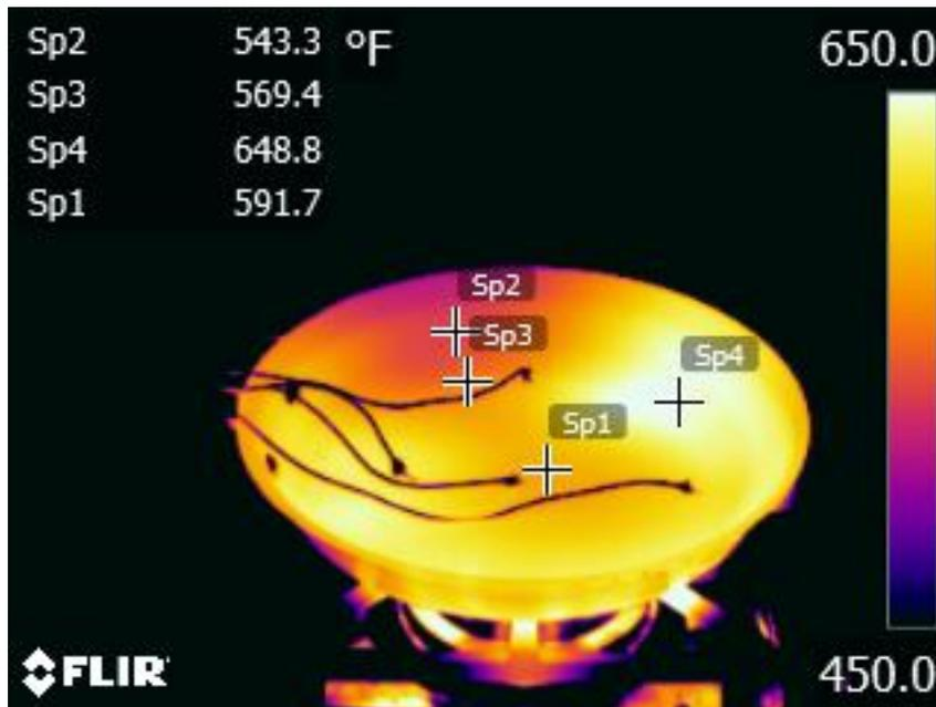
Figure 33: Temperature Profile in Aluminum Pan Power Boil (18,500 Btu/hr.)
