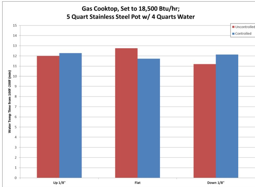
Figure 27: Water Heating Times, with and without Controls
