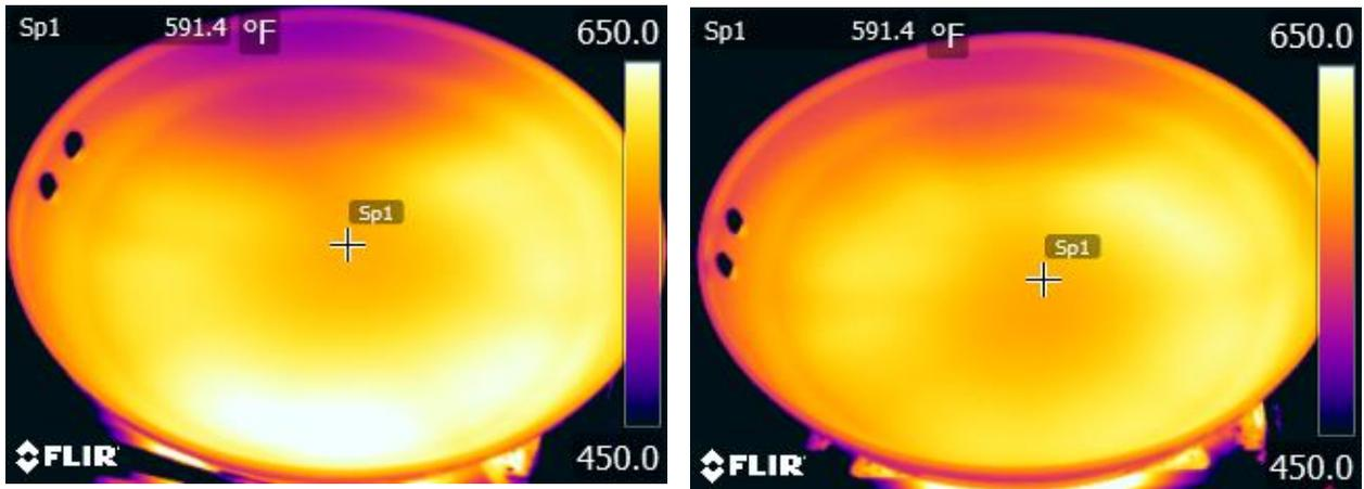
Figure 35: Comparison: Two Burner Ports Blocked (left) versus One Burner Port Blocked (right)
