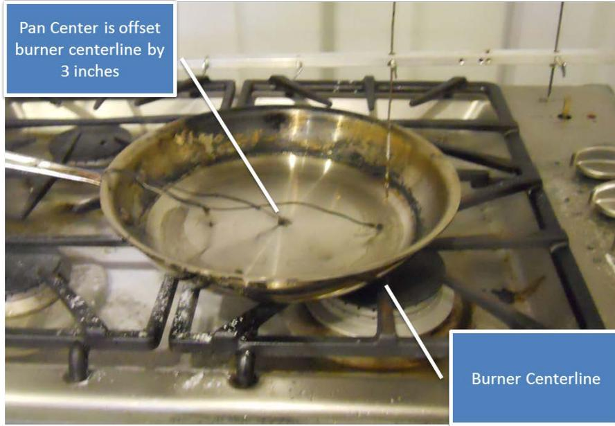
Figure 29: Pan Eccentricity Tests; 3 Inches Off the Burner Center
