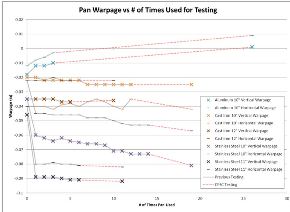
Figure 28: Pan Warpage Versus Pan Usage in Ignition Tests
