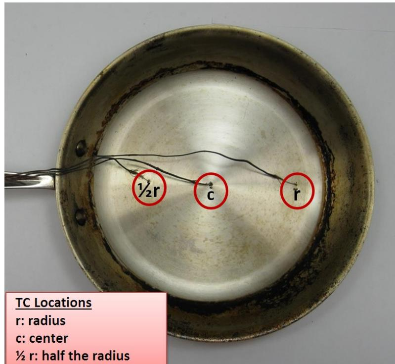
**Figure 5: Thermocouple Locations on Pan**
