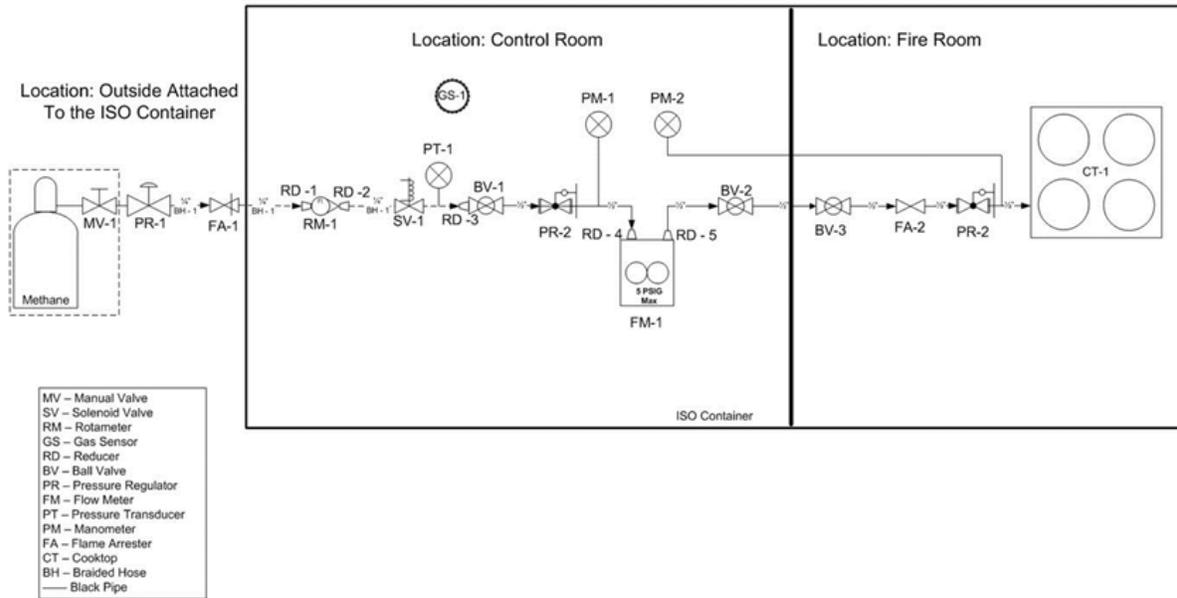
**Figure 8: Process and Instrumentation Diagram of Gas System**
