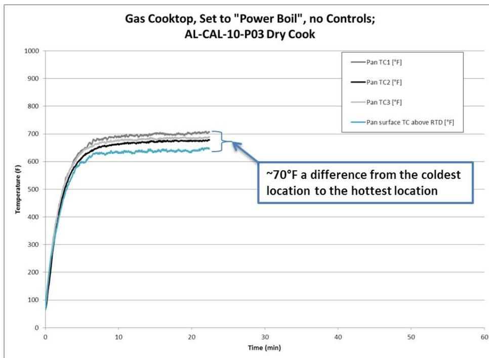
**Figure 34: Temperature Profiles from Thermocouples in Aluminum Pan on Power Boil (18,500 Btu/hr)**
