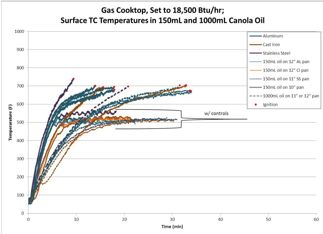
**Figure 23: Comparison of Oil Temperature Profiles for Baseline and Control System Tests (18,500 Btu/hr.)**
