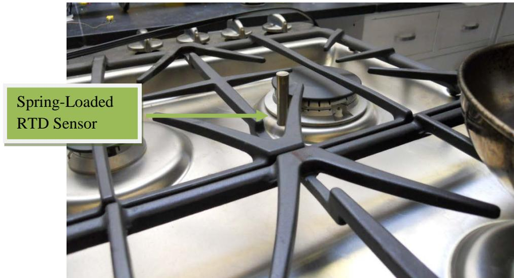
**Figure 1: RTD Sensor Integrated with the Largest Burner of the Gas Cooktop**
