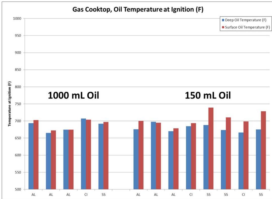
Figure 16: Baseline Testing, Oil Temperatures at Ignition
