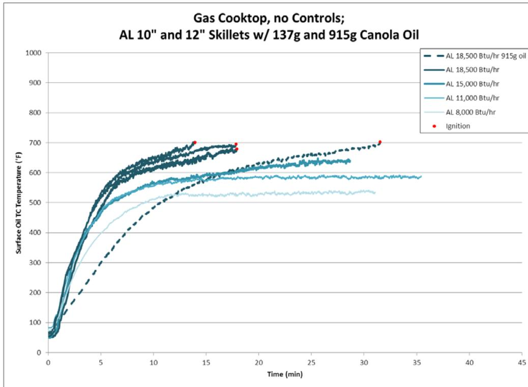
Figure 21: Surface Oil Temperature Profiles for Aluminum Pans
