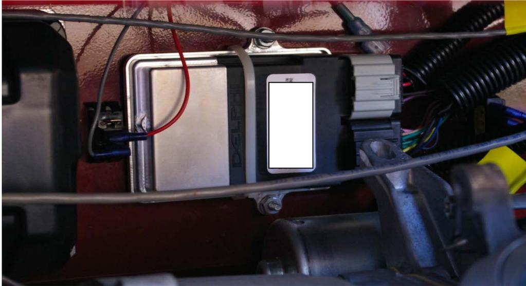
**Figure 2.4:** MT05 ECU, used in previous work, mounted inside the generator frame [6].
