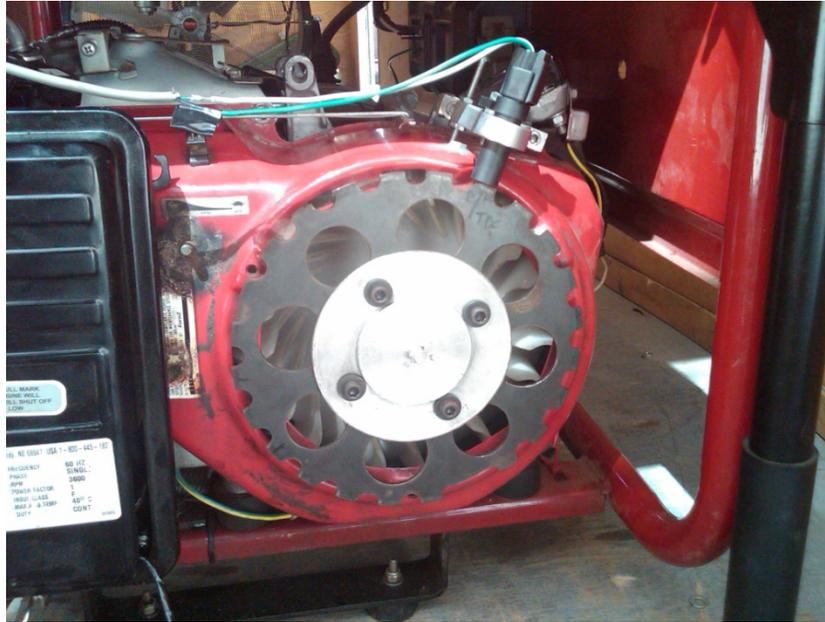
**Figure 2.1:** Crank position sensor and 24 tooth crank wheel.
