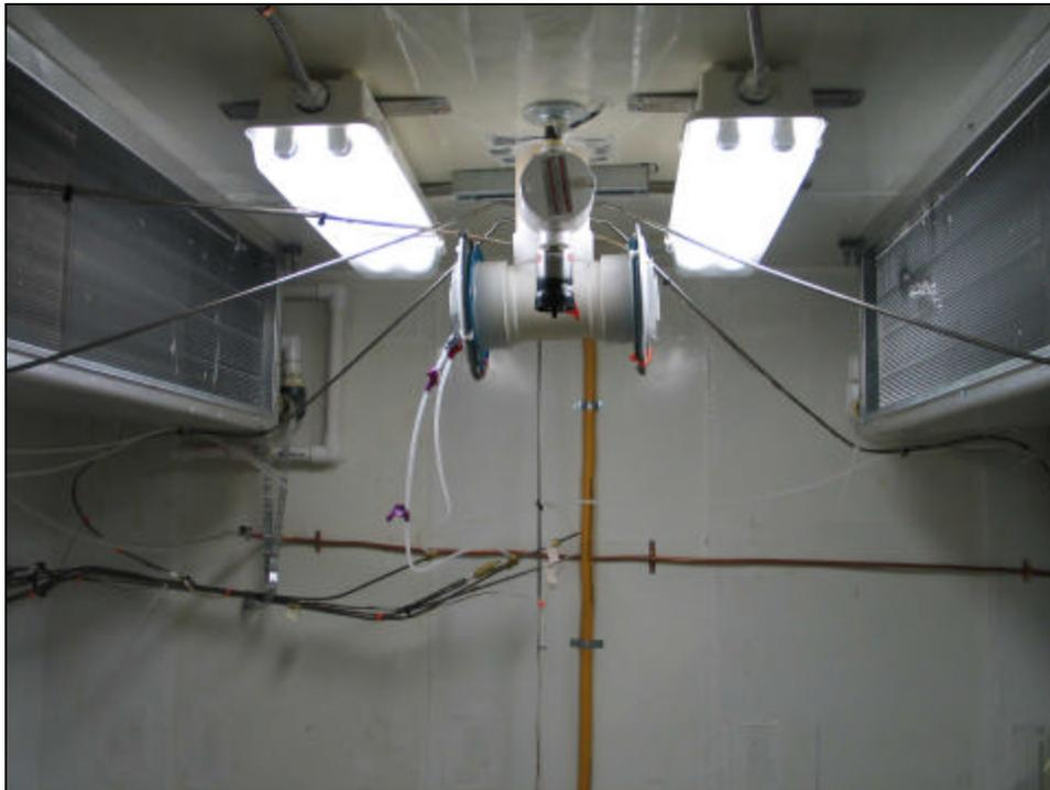
**Figure B2.** Inside view of the Medium Chamber. Air supply pipes are located at the top center of the chamber and are directed towards the heat exchangers.
